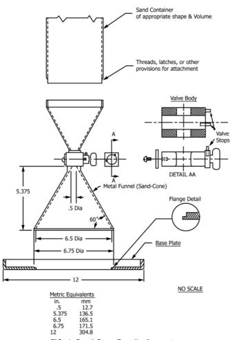
FIG. 1 Sand-Cone Density Apparatus
